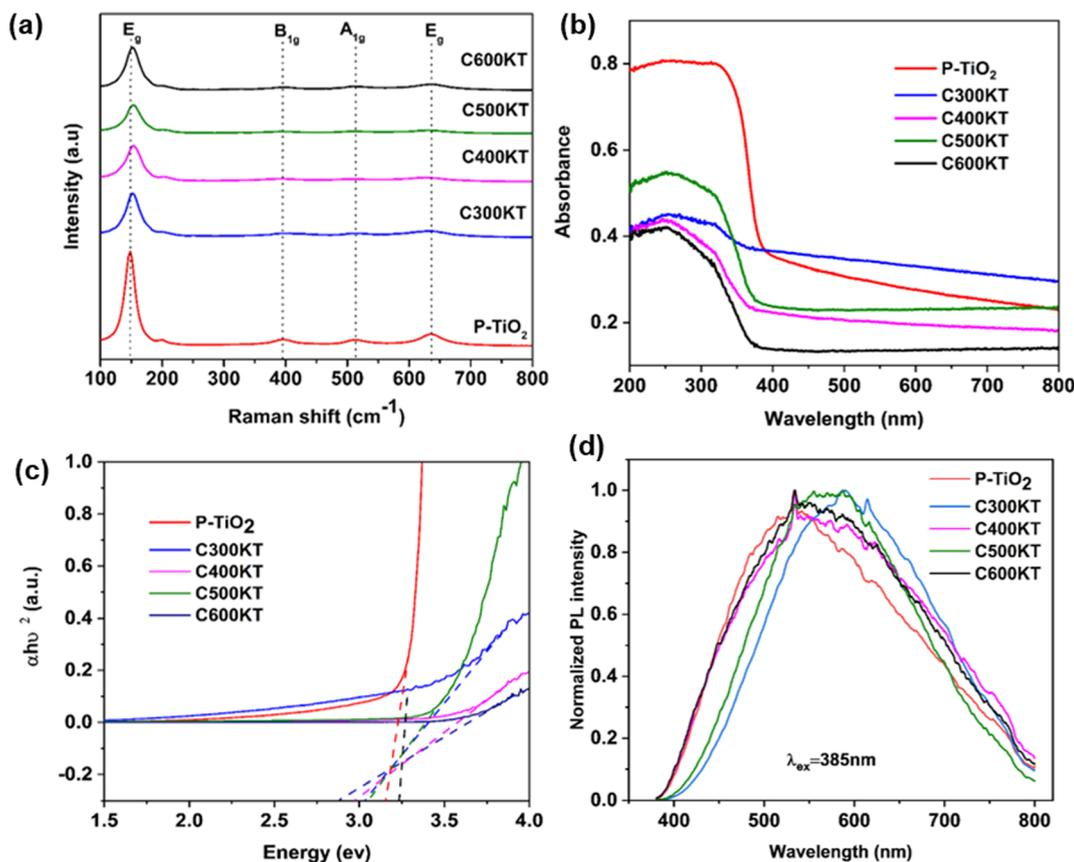
Fig. 2 (a) Raman spectra, (b) UV-vis DRS spectra, (c) Tauc plot analysis, and (d) PL spectra of P-TiO<sub>2</sub> and all NCs. Raman spectra in panel (a) are shifted vertically for clarity. Band gaps calculated from Fig. 1c are shown in Table 1.
