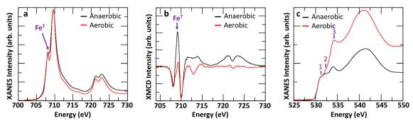
Fig. 7 (a) Comparison of Fe L<sub>2,3</sub>-edges XANES, (b) XMCD, and (c) O K-edge XANES of fresh Fh samples (2 days old) synthesized in aerobic conditions and aged in either aerobic or anaerobic conditions.
