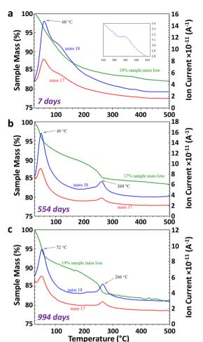
Fig. 3 TGA-MS analysis for three naturally aged Fh samples synthesized in aerobic and aged in anaerobic conditions of (a) 7 days, (b) 554 days, and (c) 994 days that shows mass loss (left y-axis) and ion current curves (right y-axis) as a function of temperature.
