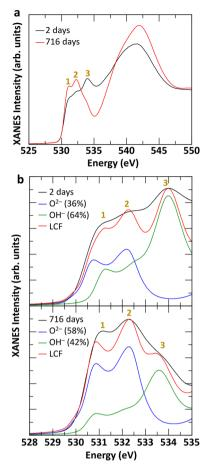
Fig. 4 (a) Comparison of the O K-edge XANES spectra for fresh (2 days) and 716 days old Fh samples synthesized in aerobic and aged in anaerobic conditions. (b) The linear combination fits (LCF) of the experimental spectra with calculated O2- and OH- contributions indicates that the peaks labelled 1 and 2 are associated with O2species, while the peak labelled 3 is associated with OH species.
