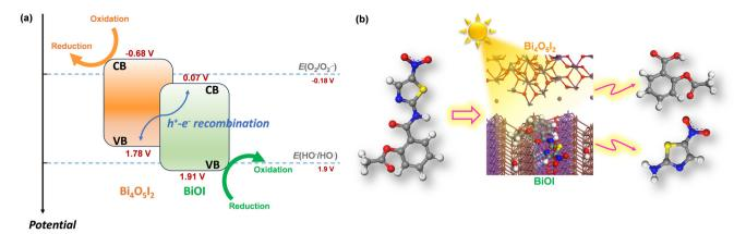
Fig. 7 (a) Band structures and redox potentials in  $BiOI/BI_4O_5I_2$  heterostructure (potentials in V vs. NHE at pH = 7) and (b) possible photodegradation pathways<sup>52</sup> of nitazoxanide by the synthesized photocatalyst.
