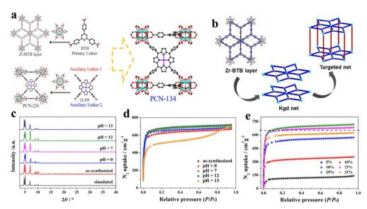
Fig. 6 Design of mixed-linker Zr-MOFs: (a) and (b) PCN-134 and PCN-224 formed by the 6-connected  $Zr_6$  cluster and TCPP. (c) The XRD patterns and (d) the  $N_2$  isotherms after immersion in aqueous solutions with different pH values at room temperature for 24 h. (e) Effects of TCPP defects of the PCN-134 system on  $N_2$  uptake measured at 77 K. Reproduced from ref. 98. Copyright 2022 ACS.
