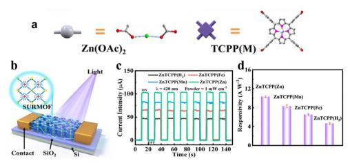
Fig. 4 (a) Preparation process of ZnTCPP(M) films. (b) Schematic diagram of ZnTCPP(M)-based photodetectors. (c) Photocurrent curve and (d) responsivity of the ZnTCPP(M)-based photodetector. Reproduced from ref. 89. Copyright 2022 ACS.
