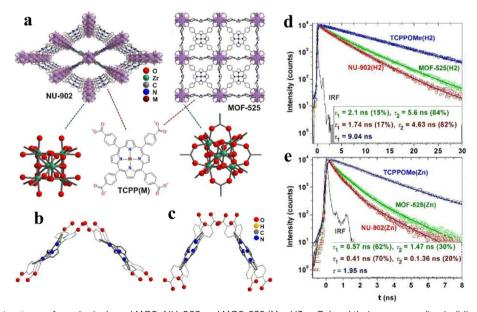
Fig. 12 (a) Molecular structures of porphyrin-based MOFs NU-902 and MOF-525 (M = H2 or Zn) and their corresponding building blocks. (b) and (c) DFT optimized structures of closely positioned porphyrin dimers in MOF-525(H2) [90°, d<sub>M-M</sub> = 13.5 Å] and NU-902(H2) [60°, d<sub>M-M</sub> = 10.5 Å]. (d) and I Transient emission decay profile for free-base and zinc(II)-metallated NU-902 and MOF-525. Reproduced from ref. 130. Copyright 2022 RSC.
