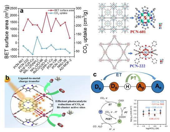
Fig. 8 (a) The BET surface area and the CO<sub>2</sub> uptake of PCN-601 and the structure of PCN-601 and PCN-222. Reproduced from ref. 113. Copyright 2022 ACS. (b) The electron-transfer mechanisms of SC-Bi-PMOFs. Reproduced from ref. 114. Copyright 2022 Elsevier. (c) The mechanisms of ET-PT and PCET and the pattern of  $log(j_{CO})$  vs.  $log(HCO_3^-)$ . Reproduced from ref. 115. Copyright 2022 Wiley.
