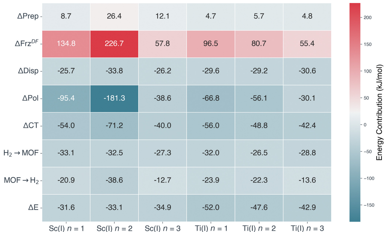
Fig. 15 Binding energies and their EDA (see eqn (2)) for the binding of three equivalents of \text{H}_2 at Sc(I) and Ti(I) sites in MFU-4l. The Sc(I) sites demonstrate a weak dependence of binding on the number of bound \text{H}_2 , which is desirable for \text{H}_2 storage purposes. By contrast, the Ti(I) sites show fall-off in binding with number of bound \text{H}_2 . See text and Fig. 16 for the origin of the remarkable change in the \Delta\text{Frz}^{\text{DF}} and \Delta\text{Pol} EDA components for the Sc(I) site with 2 bound \text{H}_2 .
