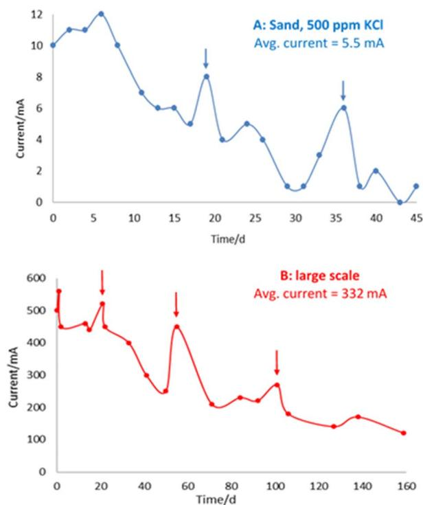
**Fig. 7** A (top) and B (bottom) – Amperometry for cell with 500 ppm KCl in sand (top, “A”) and large-scale experiment (bottom, “B”). Vertical arrows indicate addition of electrolyte and corresponding current increase. Avg. is average.
