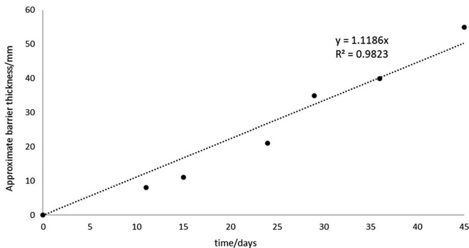
Fig. 10 Barrier growth over time, showing a strong correlation ( $R^2 = 0.98$ ) between barrier thickness and time over which voltage is applied to the system (1.25 kg sand, LWH =  $19 \times 13 \times 9$  cm cells, 500 ppm KCl electrolyte at 10 V, or  $0.53 \text{ V cm}^{-1}$ ).
