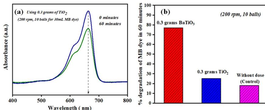
Fig. 8 (a) Absorbance spectra of MB dye using 0.3 g of  $\text{TiO}_2$  (non-piezoelectric material) in 60 min with ball milling at 200 rpm using 10 balls, (b) % degradation of MB dye in 60 min using 0.3 g of  $\text{BaTiO}_3$ ,  $\text{TiO}_2$ , and without using any catalyst in 60 min with ball milling at 200 rpm using 10 balls.
