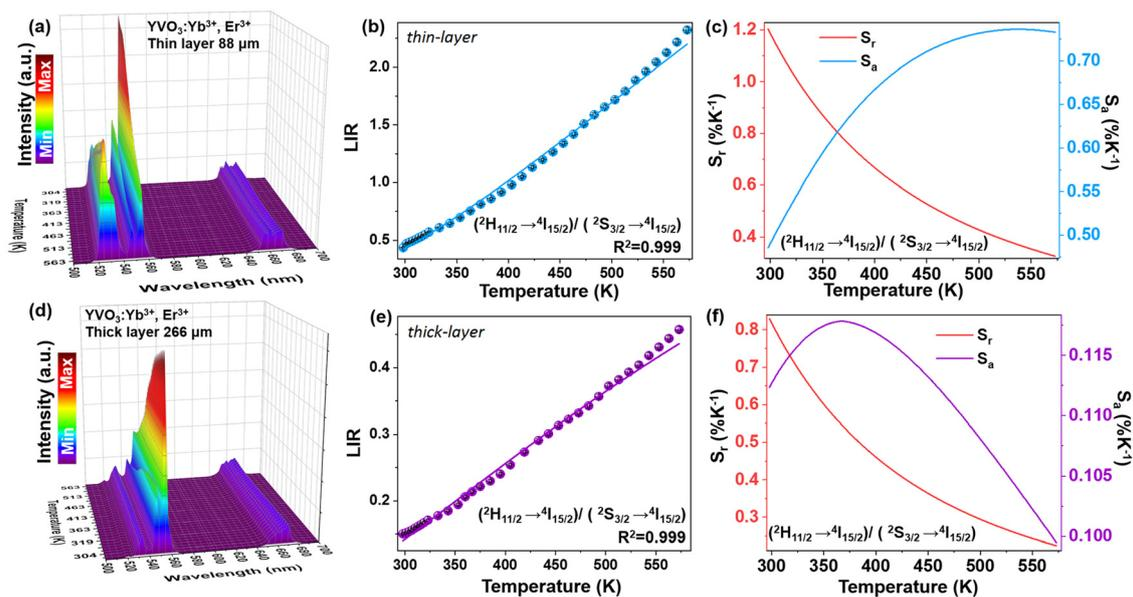
Fig. 5 (a and d) UC emission spectra of the thin-layer (a) and thick-layer (d) sample of  $\text{YVO}_4:\text{Er}^{3+}, \text{Yb}^{3+}$  nanocrystals measured at increasing temperature values ( $\lambda_{\text{ex}} = 975 \text{ nm}$ ); (b and e) the determined LIR values (525/550 nm) and (c and f) the corresponding  $S_r$  and  $S_a$  values as a function of temperature, obtained for the thin-layer (b and c) and thick-layer (e and f) samples, respectively.
