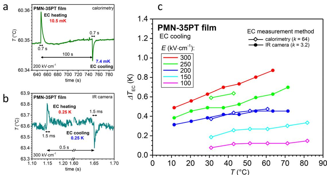
Fig. 5 Typical EC cycle obtained by (a) calorimeter method at 60.35 °C and 200  $\text{kV cm}^{-1}$  and (b) IR camera at 63.6 °C and 300  $\text{kV cm}^{-1}$ . (c) Temperature- and field-dependent  $\Delta T_{\text{EC}}$  values of the annealed PMN-35PT thick films measured by the calorimeter (open squares) and the IR camera (solid circles) methods.
