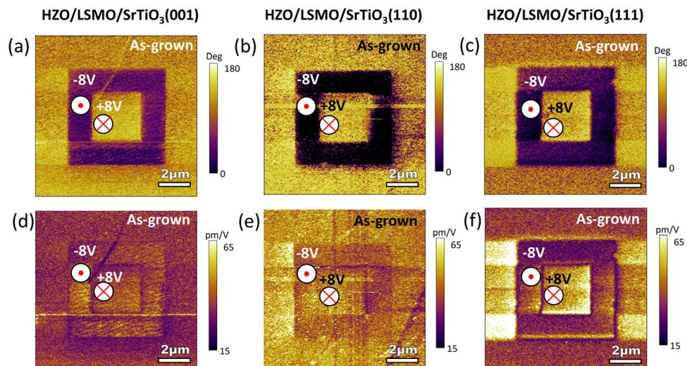
Fig. 3 (a–c) PFM out-of-plane phase images for the three HZO films grown on LSMO/SrTiO<sub>3</sub>(001), LSMO/SrTiO<sub>3</sub>(110), and LSMO/SrTiO<sub>3</sub>(111), respectively, after applying +(-)8 V in the bright (dark) regions. The outer region corresponds to the as-grown state and no voltage has been applied. (d–f) PFM out-of-plane amplitude images corresponding to the (a–c) phase image regions.
