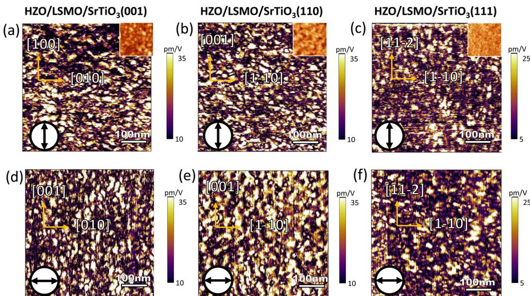
Fig. 5 (a–c) PFM in-plane amplitude images for the HZO films on LSMO/SrTiO<sub>3</sub>(001), LSMO/SrTiO<sub>3</sub>(110), and LSMO/SrTiO<sub>3</sub>(111), respectively. Response is probed along the vertical direction as indicated in the bottom-left. Top-right insets show the topography images. (d–f) Idem, while probing along the horizontal direction.
