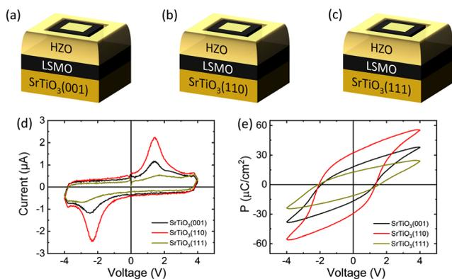
Fig. 2 (a–c) Sketch of HZO films grown on LSMO/SrTiO<sub>3</sub>(001), LSMO/SrTiO<sub>3</sub>(110), and LSMO/SrTiO<sub>3</sub>(111), respectively. (d and e) Corresponding  $I$ - $V$  and  $P$ - $V$  loops measured at 1 kHz for the three samples.
