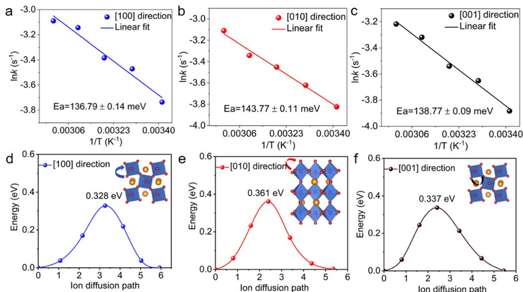
Fig. 3 (a–c) Ion migration activation energies of CsPbBr<sub>3</sub> crystal wafers along the [100], [010], and [001] directions, respectively. (d–f) Calculated energy profiles of different ionic migration paths for Br<sup>−</sup> ion vacancy along the [100], [010], and [001] orientations.
