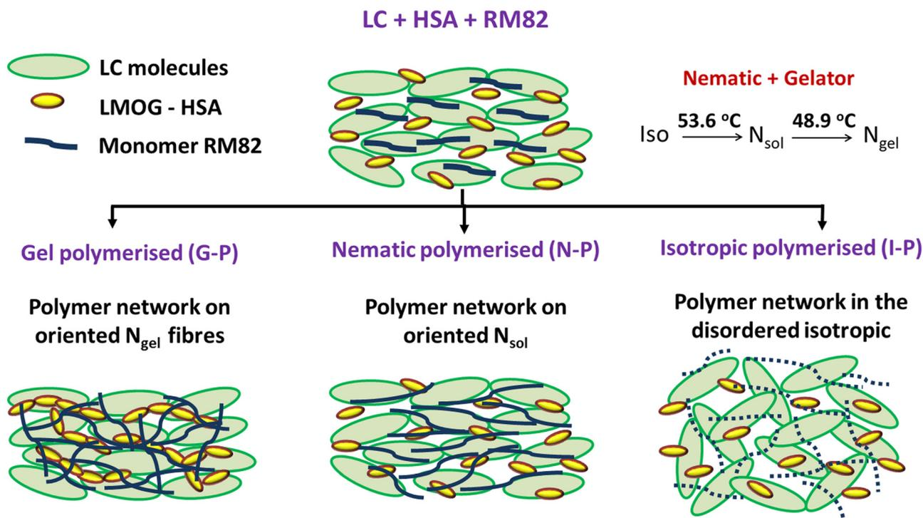
Fig. 11 Schematic of the network formation when polymerized in 3 different phases.
