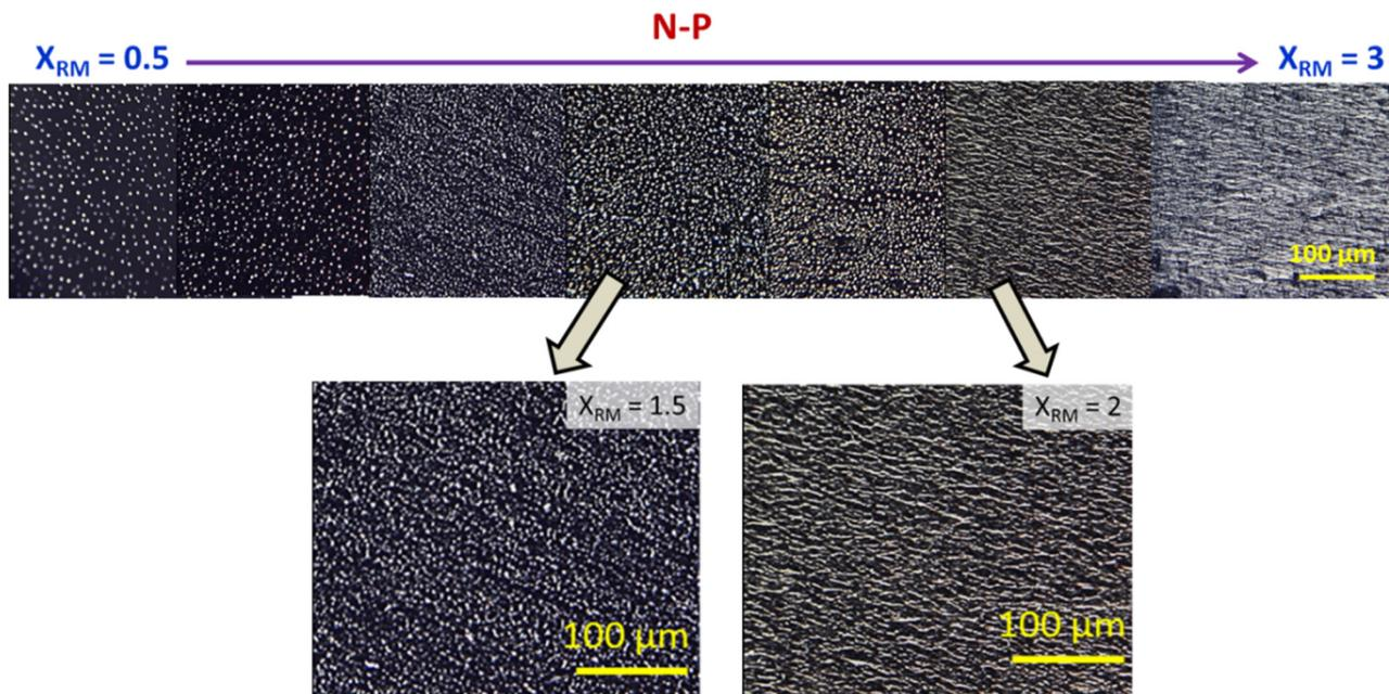
Fig. 2 POM images taken in the isotropic for samples polymerised in the nematic phase (N-P) for varied  $X_{RM}$ . While droplet morphology is seen for lower  $X_{RM}$ , as the monomer concentration increases, improved connectivity of the polymer fibres was observed. Enlarged images (below) display oriented polymer strands that are the resultant of the surrounding aligned nematic environment.
