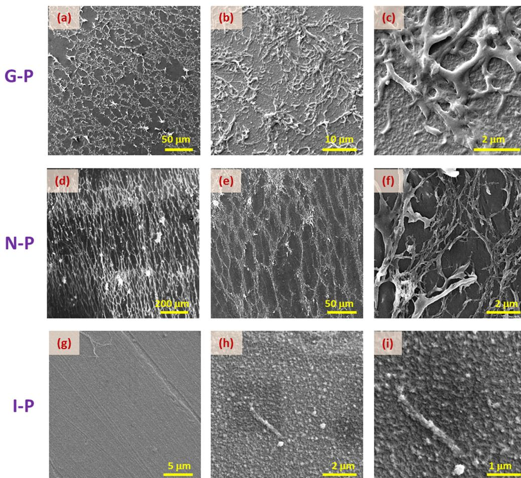
Fig. 4 SEM images depicting the polymer networks for  $X_{RM} = 3$  with magnifications of (a)  $0.5 \times 10^3$ , (b)  $3 \times 10^3$ , (c)  $20 \times 10^3$ , (d)  $0.125 \times 10^3$ , (e)  $0.5 \times 10^3$ , (f)  $15 \times 10^3$ , (g)  $5 \times 10^3$ , (h)  $15 \times 10^3$ , (i)  $30 \times 10^3$  for G-P, N-P and I-P samples shown from top to bottom, respectively.
