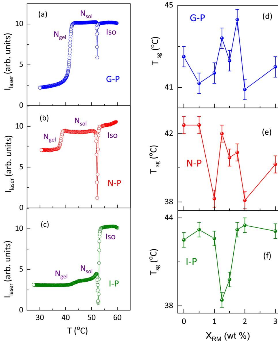
Fig. 10 Thermal variation of transmitted laser intensity ( $I_{\text{laser}}$ ) for the G-P, N-P, and I-P cases, for  $X_{\text{RM}} = 1$  in (a), (b), (c) respectively. The variation of  $T_{\text{sg}}$  with different  $X_{\text{RM}}$  is shown for the G-P, N-P, and I-P cases in (d), (e), (f), respectively.
