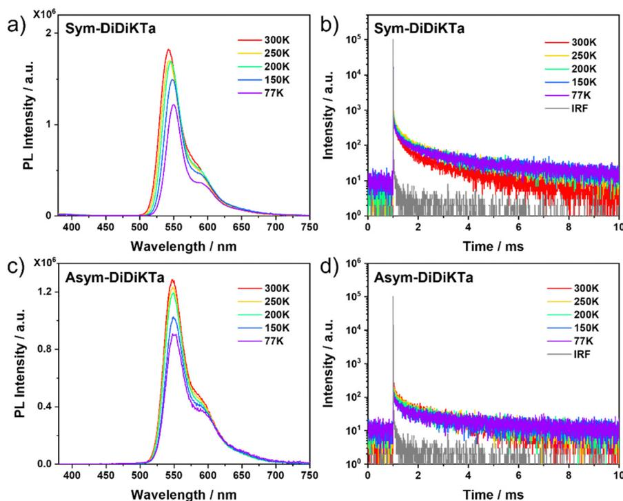
Fig. 5 (a and c) Temperature-dependent PL study of 1 wt% of **Sym-DiDiKta** and **Asym-DiDiKta**, respectively, in mCP,  $\lambda_{\text{exc}} = 350$  nm. (b and d) Temperature-dependent time-resolved PL decays for 1 wt% **Sym-DiDiKta** and **Asym-DiDiKta**, respectively, in mCP matrix ( $\lambda_{\text{exc}} = 378$  nm).
