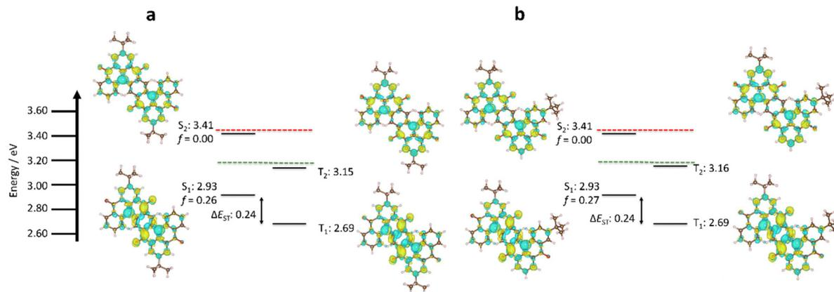
Fig. 3 Difference density picture and excited state energies of **Sym-DiDiKTA** (a) and **Asym-DiDiKTA** (b) calculated at SCS-CC2/cc-pVDZ, where red and green lines indicate  $S_1$  and  $T_1$  energies respectively of **DiKTA**, (isovalue = 0.001).
