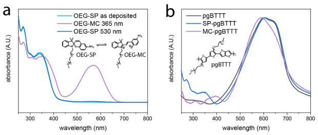
Fig. 1 UV-vis photoswitching experiments performed on thin films deposited *via* drop casting (DC) on quartz substrates. (a) Absorption spectra of **OEG-SP** in the SP and MC forms. (b) Normalised UV-vis absorption spectra of neat **pgBTTT** vs. the 20% m/m **OEG-SP/pgBTTT** blend (**SP-pgBTTT**). The spectra have been collected before (**SP-pgBTTT**) and after (**MC-pgBTTT**) irradiation with a 365 nm UV LED.
