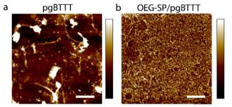
Fig. 2 Atomic force microscopy height image of thin films deposited on a UV-SiO $_2$  substate via drop casting from 0.3 mg mL $^{-1}$  CHCl $_3$  solutions. Image size:  $5 \times 5 \ \mu m^2$ . Lateral scale bar:  $5 \ \mu m$ . (a) Neat pgBTTT, Z-scale: 53 nm, nominal thickness: 60 nm,  $R_{\rm RMS}$ : 10 nm. (b) OEG-SP/pgBTTT, Z-scale: 21 nm, nominal thickness: 30 nm,  $R_{\rm RMS}$ : 3.2 nm.  $R_{\rm RMS}$  values are estimated over an area of  $2 \times 2 \ \mu m^2$ .
