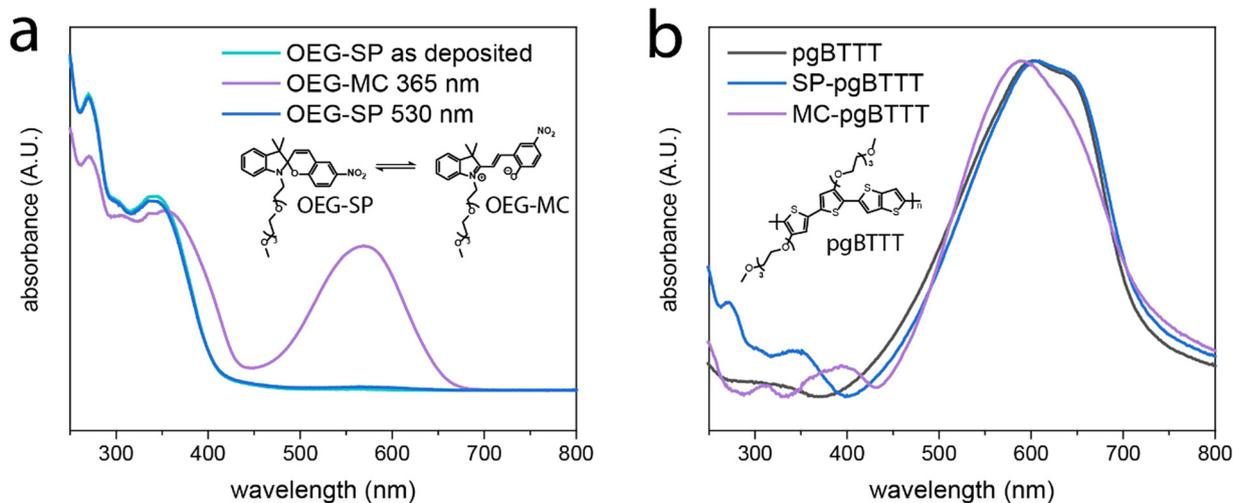
Fig. 1 UV-vis photoswitching experiments performed on thin films deposited via drop casting (DC) on quartz substrates. (a) Absorption spectra of **OEG-SP** in the SP and MC forms. (b) Normalised UV-vis absorption spectra of neat **pgBTTT** vs. the 20% m/m **OEG-SP/pgBTTT** blend (**SP-pgBTTT**). The spectra have been collected before (**SP-pgBTTT**) and after (**MC-pgBTTT**) irradiation with a 365 nm UV LED.
