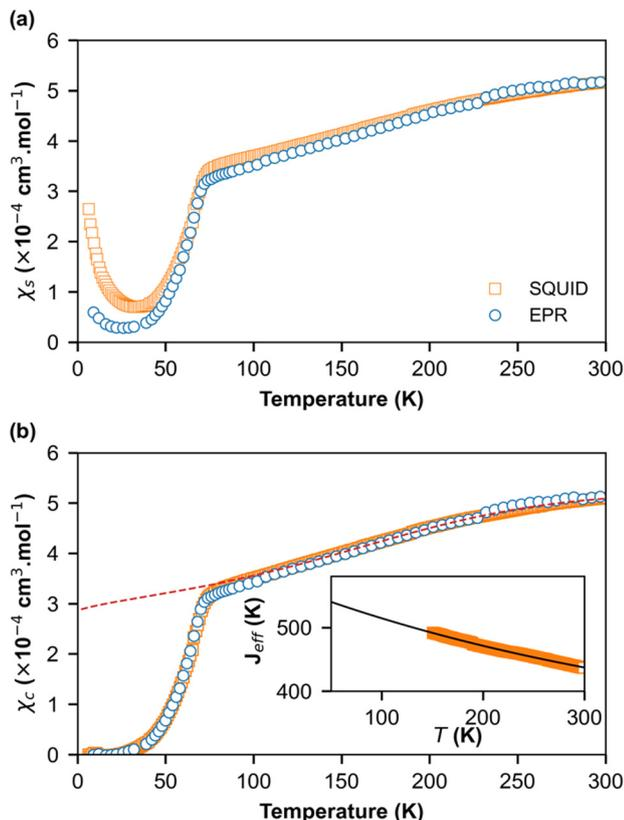
Fig. 5 (a) Temperature dependence of the spin susceptibility  $\chi_s$  deduced from ESR (circles) and SQUID (square) in  $(o\text{-DMTTF})_2\text{NO}_2$ . (b) Temperature dependence of the spin susceptibility ( $\chi_c$ ) corrected for the Curie tail of  $S = 1/2$  defects. The dashed lines are the theoretical values of susceptibility using exchange constants  $J_{\text{eff}}$  presented in the inset and extrapolated to lower temperatures.
