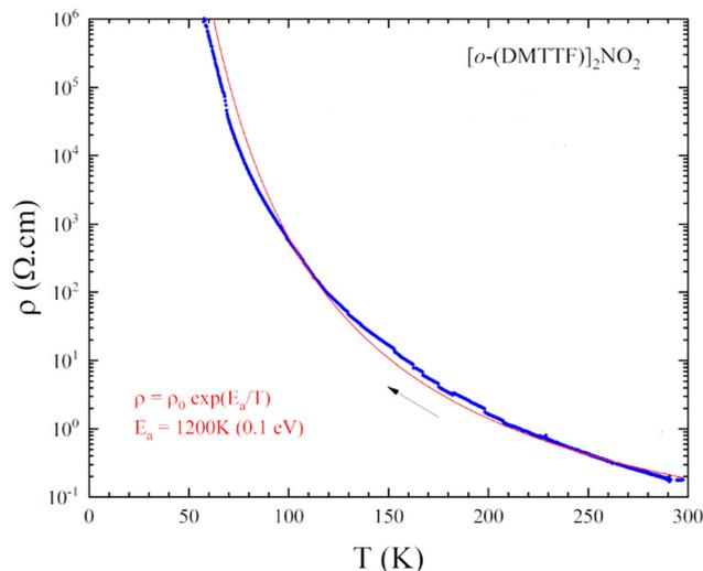
Fig. 4 Temperature dependence of the resistivity of  $(o\text{-DMTTF})_2\text{NO}_2$ .
