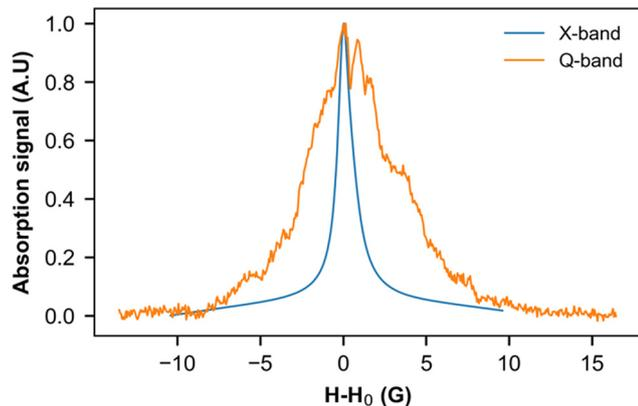
Fig. 9 EPR signal of intrinsic defects measured at 8 K in the X band (9.39 GHz) and Q band (33.75 GHz). To facilitate comparison, the resonance field  $H_0$  has been subtracted from the magnetic field.
