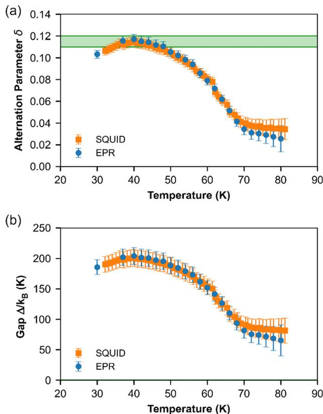
Fig. 6 Temperature dependence of (a) dimerization parameter  $\delta$  and (b) spin gap  $\Delta$  for  $(o\text{-DMTTF})_2\text{NO}_2$  extracted from ESR (circle) and SQUID (square) measurements. The green zone represents the values estimated at  $T = 0$  K with its error.
