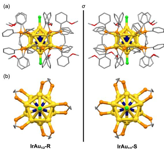
**Fig. 2** (a) SCXRD structures of **IrAu<sub>12</sub>-R** (left) and **IrAu<sub>12</sub>-S** (right). Phenyl rings, ethylene bridges, and methoxy groups are depicted as sticks and hydrogen atoms are omitted for simplicity. (b) Top view of the core structures of **IrAu<sub>12</sub>-R** (left) and **IrAu<sub>12</sub>-S** (right). Phenyl rings and methoxy groups are omitted for simplicity. Color code: yellow, Au; dark blue, Ir; orange, P; light green, Cl; red, O; gray, C.
