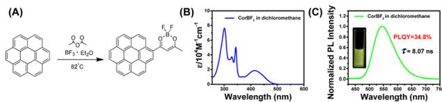
Fig. 2 (A) Cascade synthesis of luminescent  $\text{BF}_2\text{bdk}$  compounds. (B) UV-vis spectra of  $\text{CorBF}_2$  in the dichloromethane solution. (C) Steady-state emission spectra of  $\text{CorBF}_2$  in the dichloromethane solution.
