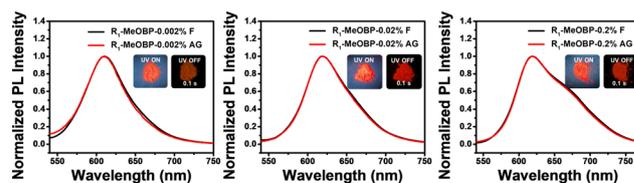
Fig. 6 The room-temperature steady-state and delayed emission (1 ms delay) spectra of R<sub>1</sub>-MeOBP afterglow materials at doping concentrations of 0.002%, 0.02% and 0.2%, respectively.
