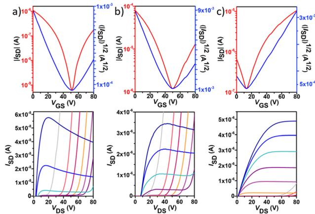
Fig. 7 Typical n-type field-effect transistor transfer (top) and output (bottom) characteristics for polymers **P2** (a), **P3** (b) and **P4** (c). The transfer characteristics were measured at a  $V_{DS}$  of 80 V. The output curves were measured at a  $V_G$  from 0 to 80 V in intervals of 10 V and over a  $V_{DS}$  range of 0 to 80 V.
