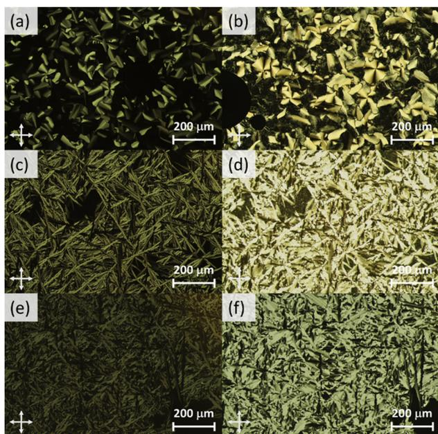
Fig. 3 Cross-polarized optical micrographs of 2 at (a) 99 °C ( $Col_h$ ) and (b) 39 °C ( $Col_h^*$ ), 3 at (c) 121 °C ( $Col_h$ ) and (d) 38 °C ( $Col_h^*$ ), and 4 at (e) 158 °C ( $Col_h$ ) and (f) 41 °C ( $Col_h^*$ ).
