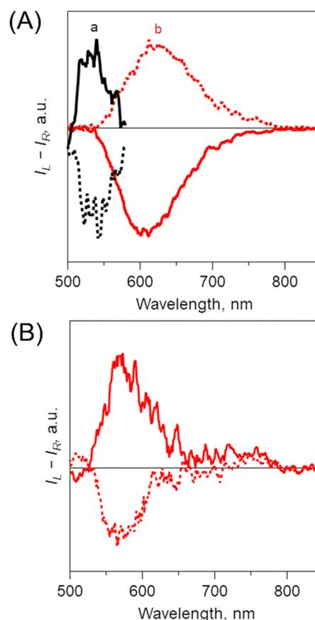
Fig. 6 (A) Circularly polarized luminescence (CPL) spectra of (a) 0Ph-B-BODIPY (monomer) in THF and (b) (0Ph-B-BODIPY)<sub>m</sub> in H<sub>2</sub>O/THF = 99/1 (v/v),  $\lambda_{\text{ex}}$ : 350 nm. (B) *R*-(1Ph-B-BODIPY)<sub>m</sub> in H<sub>2</sub>O/THF = 99/1 (v/v),  $\lambda_{\text{ex}}$ : 350 nm. Solid and dotted lines correspond to *S* and *R* forms, respectively.
