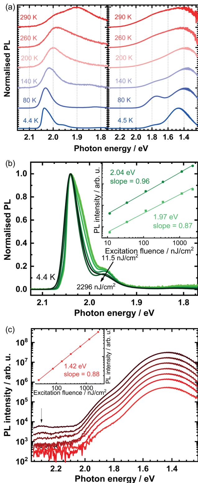
Fig. 2 (a) Temperature-dependent photoluminescence spectra of OBESnI<sub>4</sub> (left panel) and EDBESnI<sub>4</sub> (right panel). Power-dependent photoluminescence spectra at 4.4 K of (b) OBESnI<sub>4</sub> and (c) EDBESnI<sub>4</sub>, where the insets show the double-logarithmic plots of the photoluminescence intensity versus excitation fluence.
