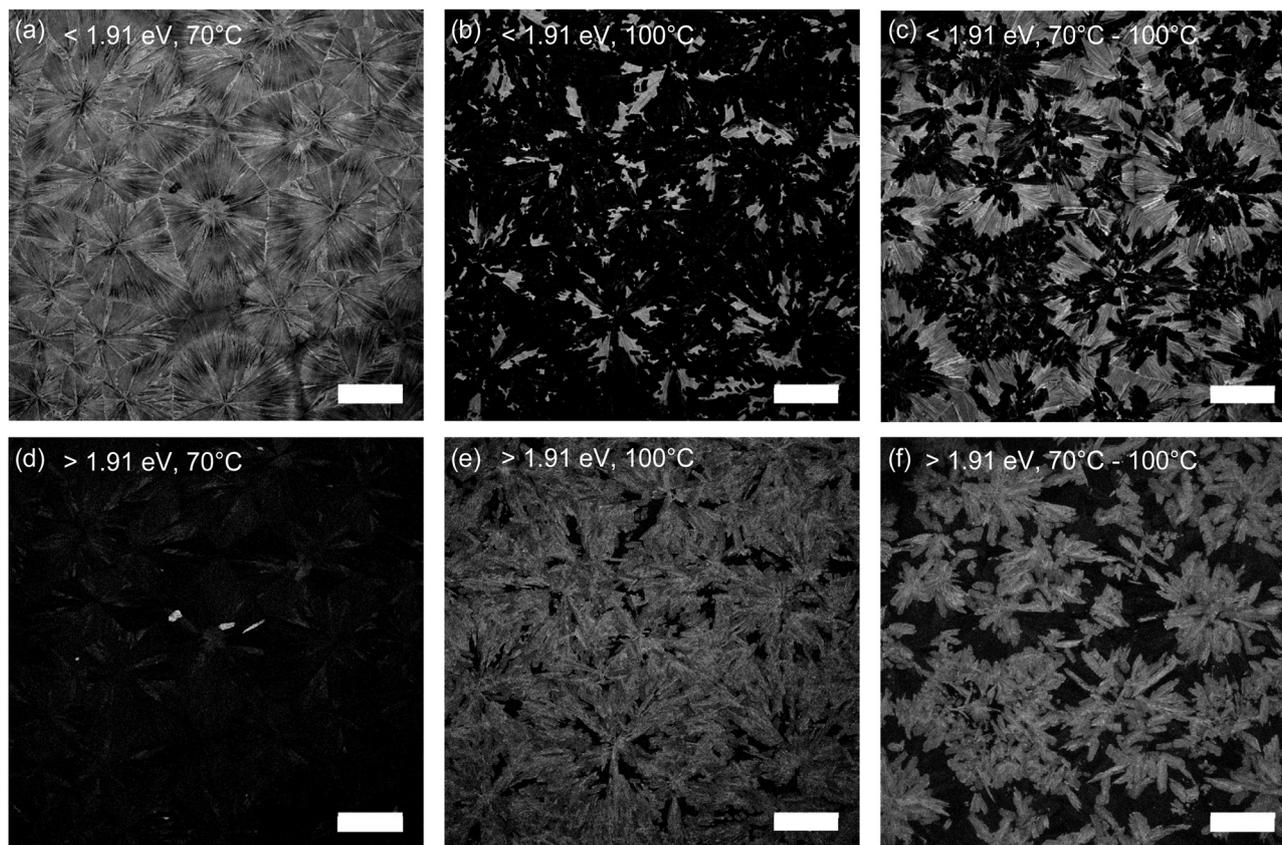
Fig. 4 Confocal photoluminescence micrographs in the range  $< 1.91\text{ eV}$  (a–c) and  $> 1.91\text{ eV}$  (d–f) for  $\text{OBESnI}_4$  thin films processed at  $70\text{ }^\circ\text{C}$ ,  $100\text{ }^\circ\text{C}$ , and  $70\text{--}100\text{ }^\circ\text{C}$ . Scale bar is  $100\text{ }\mu\text{m}$ .
