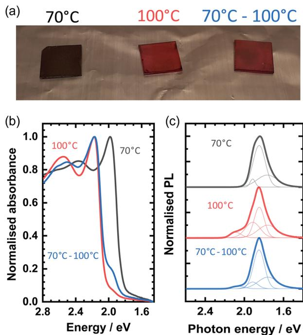
Fig. 3 (a) Optical image of OBESnI<sub>4</sub> thin films processed at 70 °C, 100 °C, and 70–100 °C. (b) Absorbance spectra and (c) photoluminescence spectra of the thin films.
