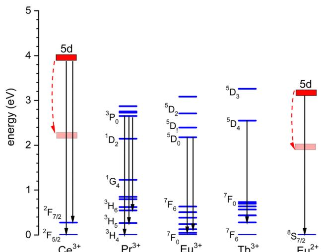
Fig. 2 Relevant level energies and luminescence transitions of  $\text{Ce}^{3+}$ ,  $\text{Pr}^{3+}$ ,  $\text{Eu}^{3+}$ ,  $\text{Tb}^{3+}$ , and  $\text{Eu}^{2+}$ . The energy of the lowest  $5d$ -level depends on the compound and the range is indicated by the curved dashed arrows.
