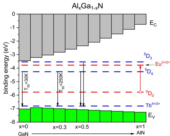
Fig. 9 Stacked VRBE scheme of the  $\text{Al}_{1-x}\text{Ga}_x\text{N}$  system with the  $\text{Tb}^{3+}$  ground and excited state levels. The  $\text{Eu}^{3+}$  ground and excited  $5\text{D}_0$  levels are drawn as hole states.
