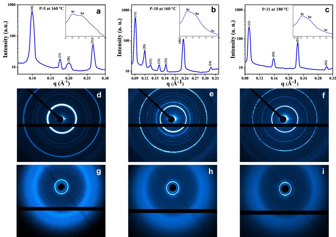
Fig. 4 Small- and wide-angle (inset) X-ray diffraction patterns of the Col phases formed by compounds (a) **P-5** at 160 °C ( $\text{Col}_h$ ), (b) **P-10** at 160 °C ( $\text{Col}_{ob}$ ) and (c) **P-11** at 180 °C ( $\text{Col}_r$ ) upon cooling ( $h_r$ , cholesterol–cholesterol correlation;  $h_a$ , alkyl chain–chain correlation;  $h_c$ , disc–disc correlation). The lower panels show the respective 2D SAXS (d–f) and WAXS (g–i) diffraction patterns for the compounds in (a–c).
