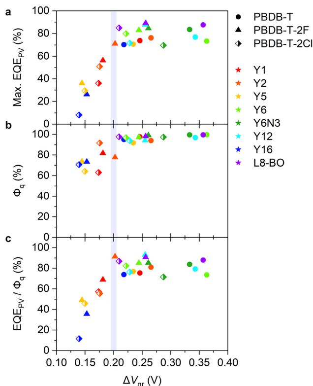
Fig. 3 (a) Maximum EQE<sub>PV</sub>, (b) PL quenching yield  $\Phi_q$ , and (c) EQE<sub>PV</sub>/ $\Phi_q$  plotted against  $\Delta V_{nr}$ .
