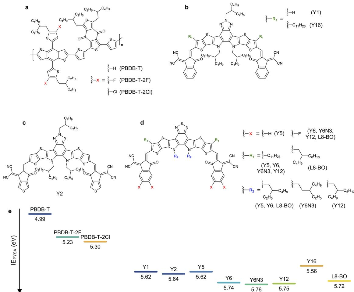
**Fig. 1** Chemical structures of (a) donor and (b–d) acceptor materials employed in this study. PBDB-T-2F and PBDB-T-2Cl are also referred to as PM6 and PM7, respectively. (e) Ionization energies (IEs) of pristine donor and acceptor films determined by photoelectron yield spectroscopy in air (PYSA).
