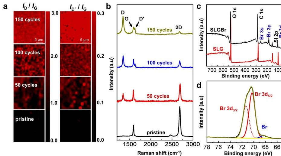
Fig. 2 (a) Raman mapping of the intensity ratio  $I_D/I_G$  and  $I_{D'}/I_G$  with the same scale bar. (b) The corresponding Raman spectra of SLG with different degrees of bromination. (c) XPS spectrum of SLG and SLGBr before and after bromination. (d) High-resolution XPS spectrum of Br 3d in SLGBr.
