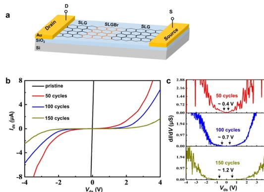
Fig. 3 (a) The illustration of a typical SLG/SLGBr/SLG diode. (b) The  $I_{ds}$ - $V_{ds}$  curves of SLG/SLGBr/SLG diodes with different degrees of bromination. (c) The corresponding differential conductance  $dI/dV$  as a function of  $V_{ds}$  for the diodes.
