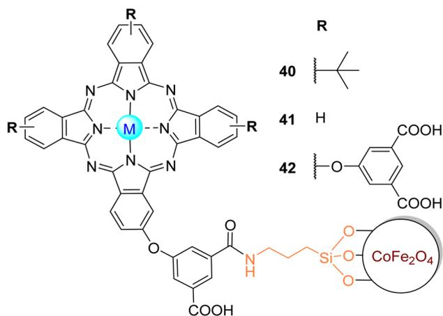
Fig. 12 Zn40–Zn42 coupled to CoFe<sub>2</sub>O<sub>4</sub> MNP used by Nyokong and co-workers<sup>142,143</sup> for the degradation of MO.
