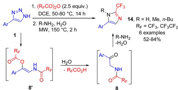
Scheme 11 One-pot synthesis of 2-fluoroalkyl-imidazoles from NH-1,2,3-triazoles.
