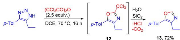
Scheme 9 Formation of 2-unsubstituted oxazole from NH-1,2,3-triazole and trichloroacetic anhydride.
