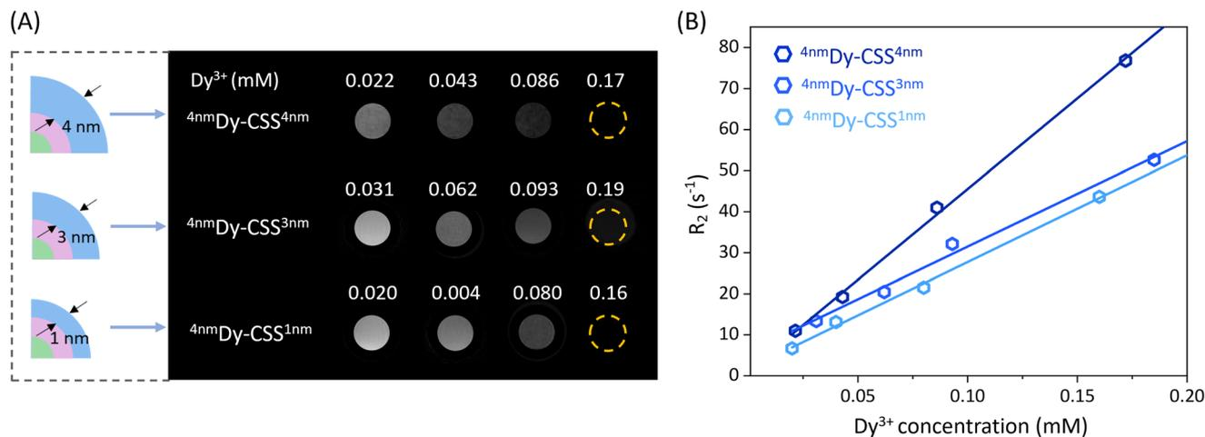
**Fig. 3** (A)  $T_2$ -Weighted MR images of Cit-Dy-CSS NPs with varying NaDyF<sub>4</sub> outer shell thickness (Cit-<sup>4nm</sup>Dy-CSS<sup>1nm</sup>, Cit-<sup>4nm</sup>Dy-CSS<sup>3nm</sup> and Cit-<sup>4nm</sup>Dy-CSS<sup>4nm</sup>) as a function of the Dy<sup>3+</sup> concentration. (B) Relaxation rate  $R_2$  ( $=1/T_2$ ) of water protons plotted against the molar concentration of Dy<sup>3+</sup> at 7 T. Solid lines are linear fits.
