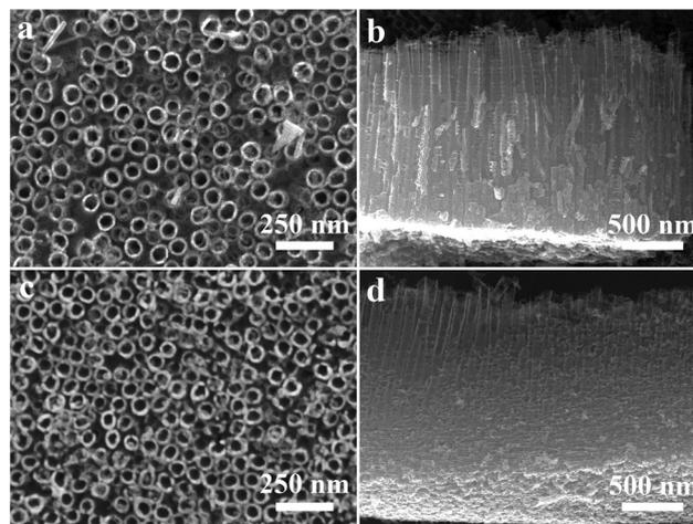
Fig. 1 SEM images of the surface and cross-section of TNTA (a and b) and Ru-TNTA (c and d).
