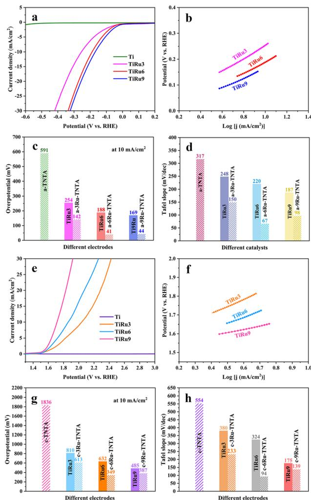
**Fig. 10** HER performance of TiRux (a and b) and the comparison histogram with a-*x*Ru-TNTA (c and d) and OER performance of TiRux (e and f) and the comparison histogram with c-*x*Ru-TNTA (g and h).
