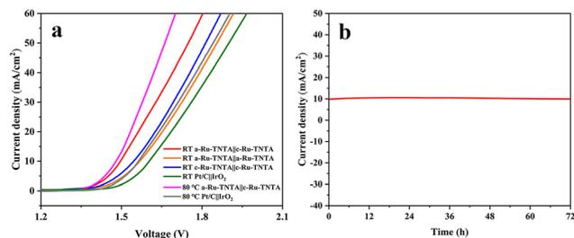
**Fig. 13** Current density vs. voltage curves for water splitting with different cathodes and anodes (a) and stability of the a-Ru-TNTA|c-Ru-TNTA electrode group (b).
