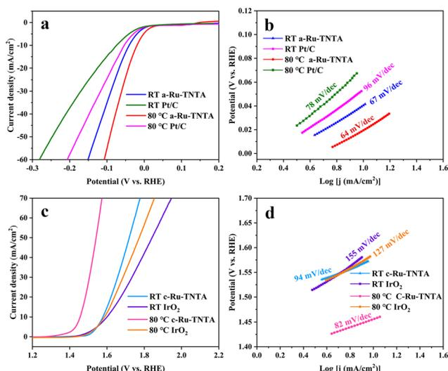
**Fig. 12** HER performances of a-Ru-TNTA and commercial Pt/C (a and b) and OER performances of c-Ru-TNTA and  $\text{IrO}_2$  (c and d) at room temperature and  $80 \text{ }^\circ\text{C}$  test temperature.
