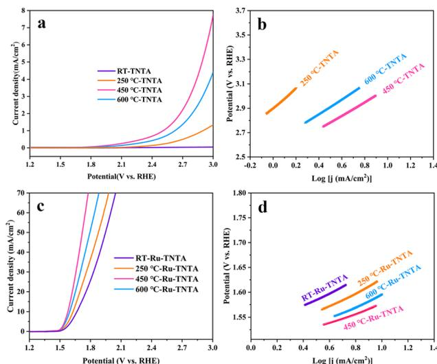
Fig. 7 OER performances of TNTA (a and b) and Ru-TNTA (c and d) annealed at different temperatures.
