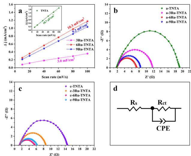
Fig. 9 The current density vs. sweep speed curves of *x*Ru-TNTA (a), Nyquist plots of *a*-*x*Ru-TNTA for the HER (b) and *c*-*x*Ru-TNTA for the OER (c) and the respective equivalent circuits used to fit the data (d).
