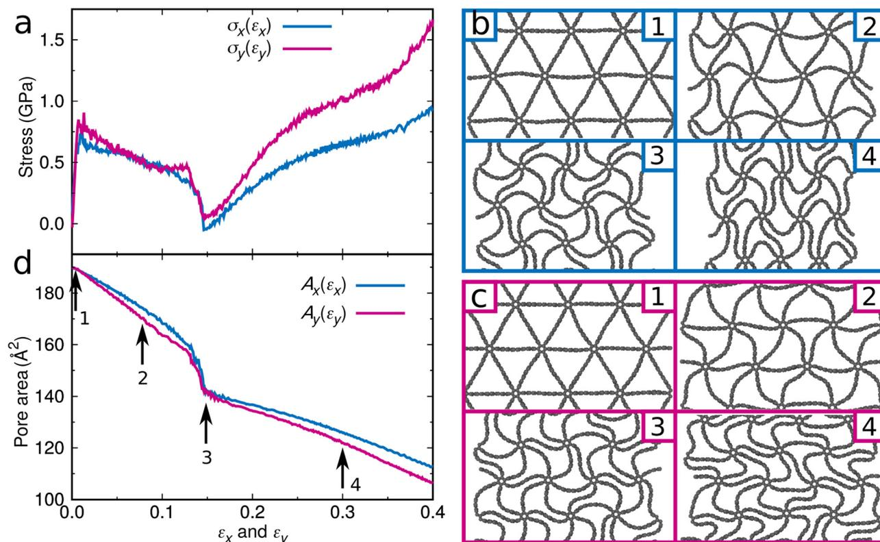
Fig. 2 Graphene foam membrane with an initial pore area of 187 Å<sup>2</sup>: (a) Stress-strain curves for loading in the *x*- and *y*-directions. Structure under increasing strain (0.005, 0.075, 0.150, and 0.300) applied in the (b) *x*- and (c) *y*-directions. (d) Pore area as a function of the strain applied in the *x*- and *y*-directions.
