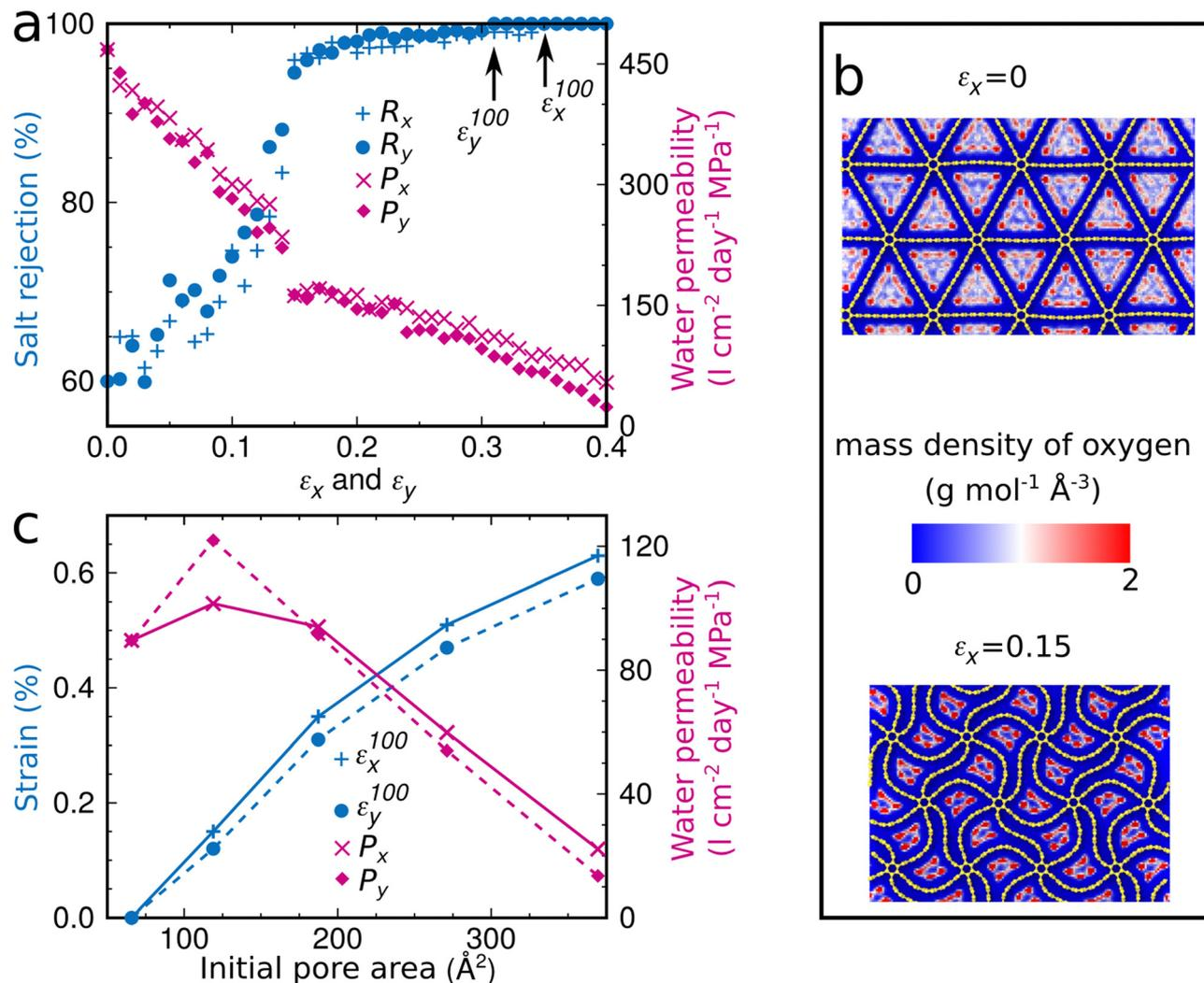
Fig. 4 (a) Salt rejection and water permeability as a function of the strain applied in the *x*- and *y*-directions for an initial pore area of 187 Å<sup>2</sup>. (b) Effect of the strain applied in the *x*-direction on the mass density of oxygen inside the pores for an initial pore area of 187 Å<sup>2</sup>. (c) Applied strain required for perfect salt rejection and corresponding water permeability as a function of the initial pore area.
