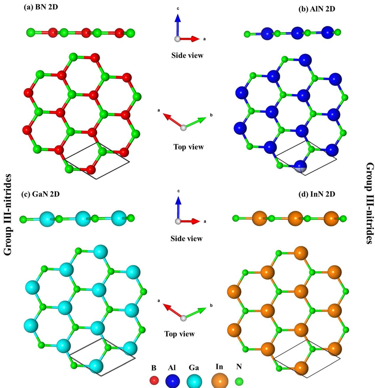
**Fig. 1** (a–d) Side view and top view for BN, AlN, GaN, and InN monolayers, respectively. The solid black is a unit cell with two atoms. The red, blue, cyan, yellow, and green balls represent by B, Al, Ga, In, and N atoms.
