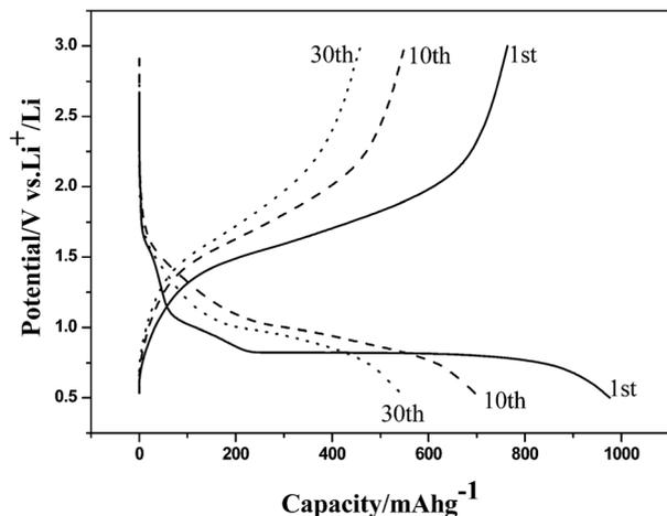
Fig. 19 The first (solid line), 10th (dashed line), and 30th (dotted line) charge–discharge curves of flower-like  $\alpha$ -Fe<sub>2</sub>O<sub>3</sub> nanostructures at a current density of 0.2 mA cm<sup>-2</sup>. Reprinted with permission from ref. 306. Copyright © 2008, American Chemical Society. All rights reserved.
