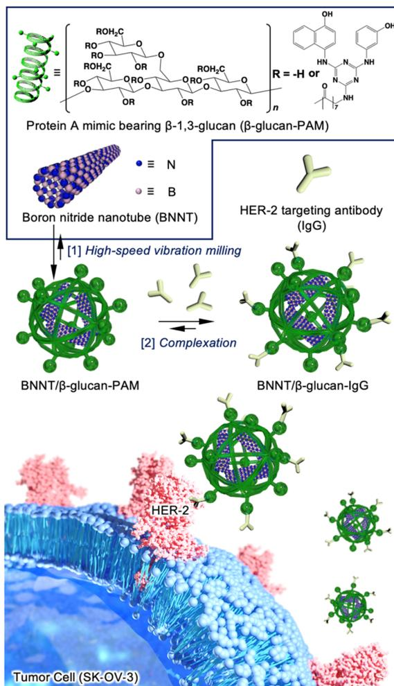
**Fig. 1** Schematic illustration of the two-step method used to prepare the tumor-selective BNNT/β-glucan complex conjugated to a HER-2-targeting antibody (BNNT/β-glucan-IgG). [1] A boron nitride nanotube and a Protein A mimic bearing β-1,3-glucan (β-glucan-PAM) were complexed *via* the facile HSVM method. [2] The HER-2-targeting antibody was conjugated to BNNT/β-glucan using the binding ability of the Protein A mimic moiety.
