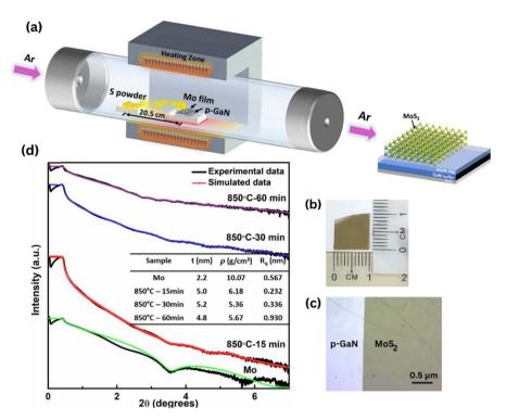
Fig. 1 (a) Schematic illustration of the CVD setup. (b) Photograph image of the MoS<sub>2</sub> film deposited on 1 cm  $\times$  1 cm p-GaN. (c) Optical image of the large-area patterned MoS<sub>2</sub> film grown on p-GaN through a shadow mask, taken at 20× magnification. (d) X-ray reflectivity curve of the asgrown Mo and MoS $_2$  films deposited on p-GaN at 850 °C - 15 min, 850 °C - 30 min and 850 °C - 60 min.
