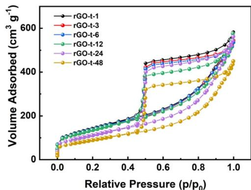
Fig. 3 Nitrogen adsorption/desorption isotherms of rGO synthesized with different reduction times (1 h, 3 h, 6 h, 12 h, 24 h, and 48 h).
