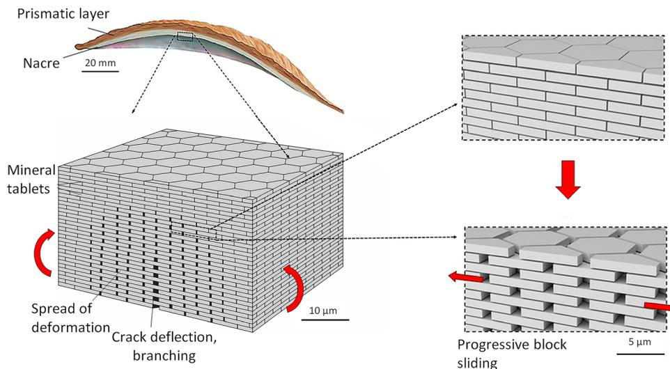
**Fig. 1** Schematic of Nacre's brick-wall architecture and the prevailing toughening mechanisms. Reproduced from ref. 4 and 10 with permission from Springer Nature, copyright 2020, and the American Association for the Advancement of Science, copyright 2019.
