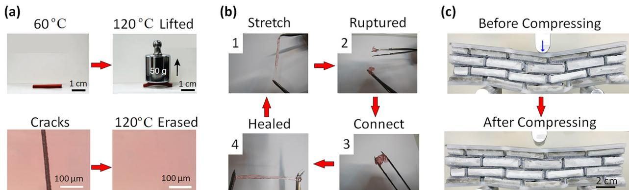
**Fig. 8** Self-healing behaviours with (a) a nacre-like architecture based on a dynamic polymer network, (b) the UPy-units doped OEGMA copolymers, and (c) nacre-inspired cement-like materials. Image (a) is adapted from ref. 49. Images (b) and (c) are reproduced from ref. 101 and 24 with permissions respectively from WILEY-VCH Verlag GmbH & Co. KGaA, Weinheim, copyright 2015 and from Elsevier Ltd, copyright 2021.
