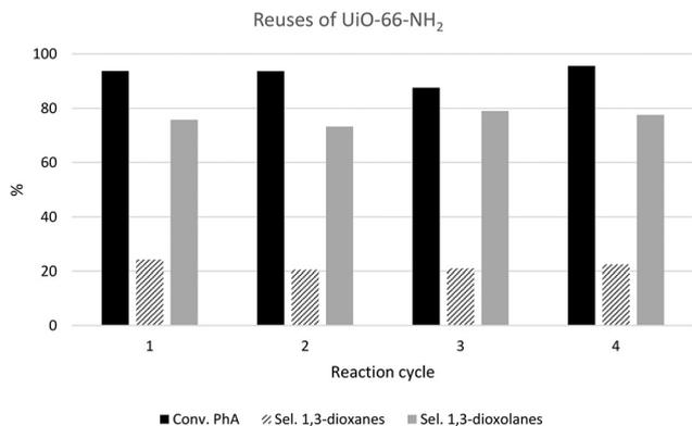
**Fig. 8** Results of the consecutive reuses of the UiO-66-NH<sub>2</sub>-18 sample in the acetalization reaction of phenylacetaldehyde with glycerol after 6 h.
