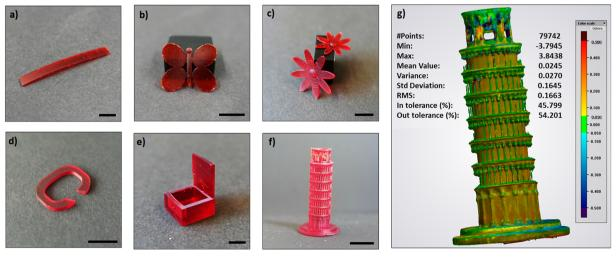
Fig. 2 3D printed structures using the formulation containing AzoCl: a) stripe, b) butterfly, c) flower, d) chain segment e) box, f) Pisa tower. g) Structural fidelity achieved demonstrated by the printed Pisa tower structure: heat map illustrating deviations between the 3D scanned image of the printed structure with its STL file. Scale bar = 10 mm.
