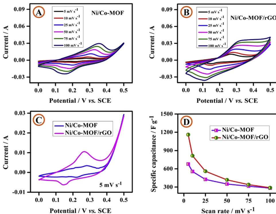
**Fig. 17** Cyclic voltammetric curves of (A) Ni/Co-MOF and (B) the Ni/Co-MOF/rGO composite at various scan rates; (C) cyclic voltammetric curves of Ni/Co-MOF and the Ni/Co-MOF/rGO composite at a scan rate of  $5 \text{ mV s}^{-1}$  and (D) specific capacitance vs. scan rate. Reproduced from ref. 171 with permission from Elsevier Ltd, Copyright 2020.
