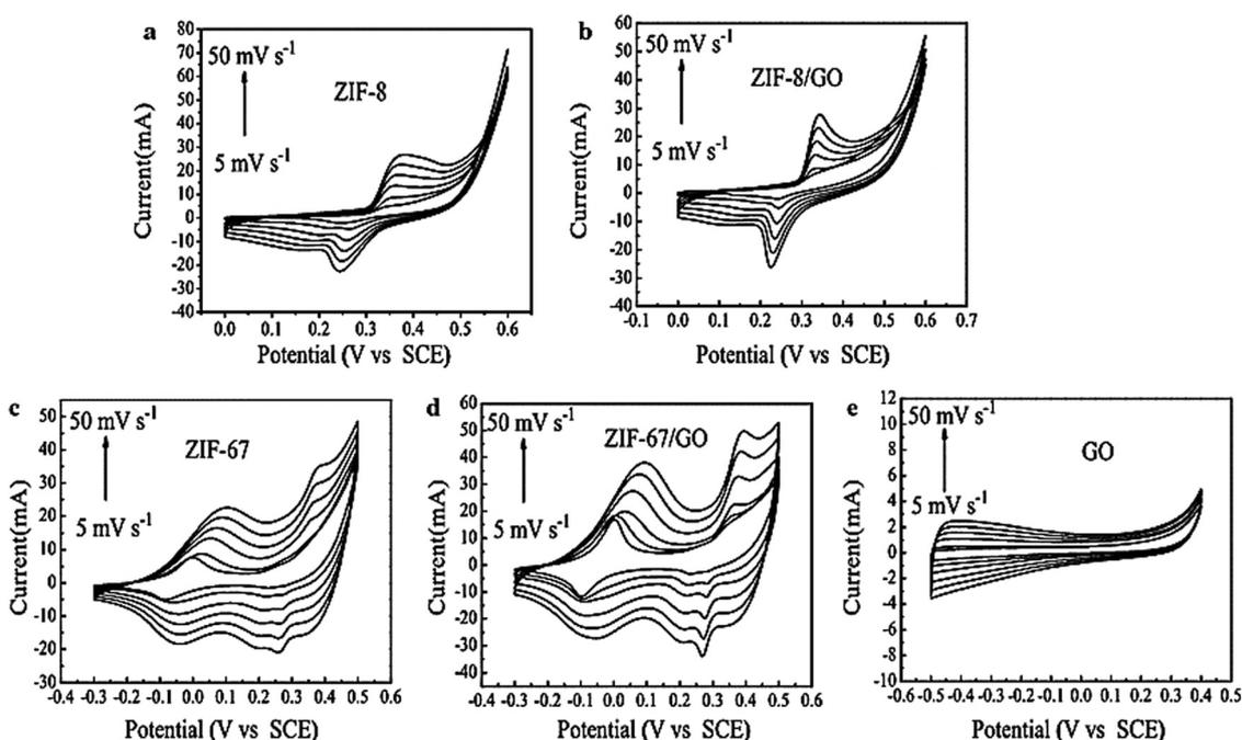
Fig. 12 Cyclic voltammograms of (a) ZIF-8, (b) ZIF-8/GO, (c) ZIF-67, (d) ZIF-67/GO, and (e) GO at increasing voltage scan rates of 5, 10, 20, 30, 40, and 50 mV s<sup>-1</sup>. Reproduced from ref. 161 with permission from Springer Science, Copyright 2016.
