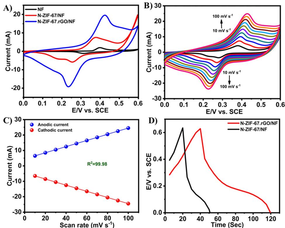
Fig. 14 CV curves of bare NF, N-ZIF-67/NF, and N-ZIF-67.rGO/NF in 2 M KOH with a scan rate of  $50 \text{ mV s}^{-1}$  (A), CV curves of N-ZIF-67.rGO/NF in 2 M KOH at different scan rates (B), anodic and cathodic peak currents for N-ZIF-67.rGO/NF as a function of scan rate (C), and GCD curves of N-ZIF-67/NF and N-ZIF-67.rGO/NF in 2 M KOH at a current density of  $20 \text{ mA cm}^{-2}$  (D). Reproduced from ref. 164 with permission from American Chemical Society, Copyright 2021.
