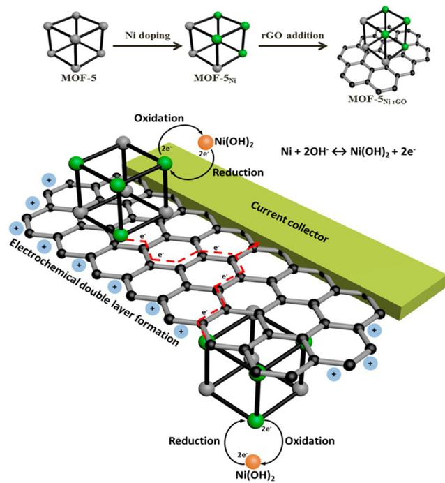
**Scheme 3** The concept for Ni doping and incorporating rGO to form a composite of rGO and Ni-doped MOF-5 and its use as an electrode material that harnesses both the electrochemical double layer performance of rGO and the reversible redox reactions of Ni metal centres with a synergy that facilitates effective and efficient charge transfer processes. Reproduced from ref. 165 with permission from American Chemical Society, Copyright 2015.
