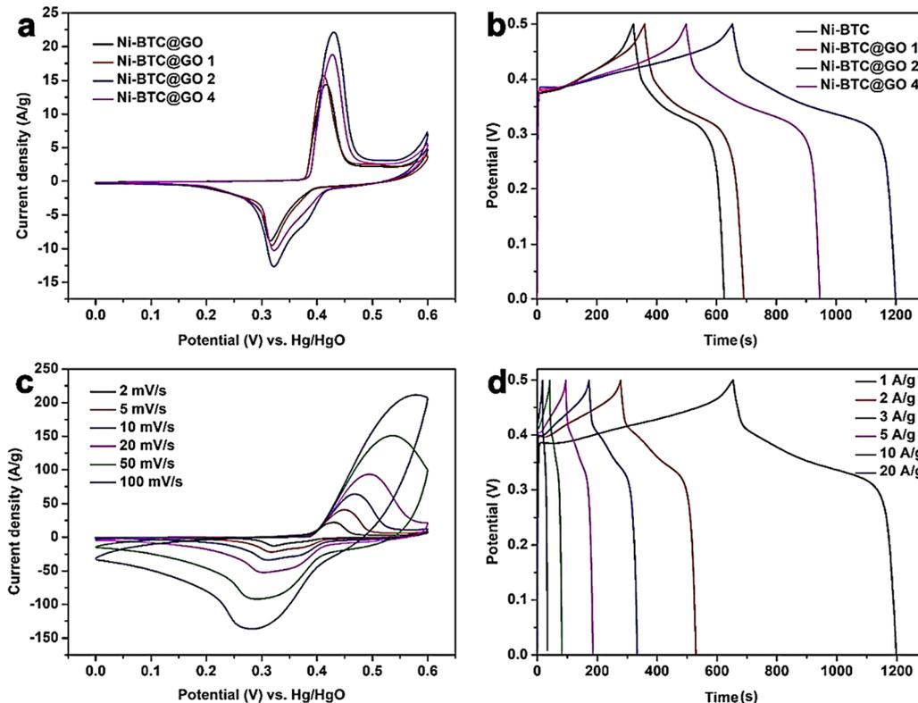
Fig. 8 (a) CV curves of Ni-BTC and Ni-BTC@GO composites at 2 mV s<sup>-1</sup>, (b) GCD curves of Ni-BTC and Ni-BTC@GO composites at 1 A g<sup>-1</sup>, (c) CV curves of Ni-BTC@GO 2 at 2–100 mV s<sup>-1</sup>, and (d) GCD curves of Ni-BTC@GO 2 at 1–20 A g<sup>-1</sup>. Reproduced from ref. 151 with permission from American Chemical Society, Copyright 2023.
