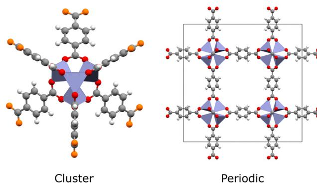
**Fig. 2** Cluster and unit cell representations of MOF-5 (Zn: blue, C: grey, O: red, H: white). Periodic codes perform calculations on the repeating unit cell in a PW basis set, whereas molecular codes perform calculations on clusters, in a GTO basis set. The outer oxygen atoms (orange) of the cluster are one half of a bond cut; these dangling bonds must be saturated using a capping scheme.
