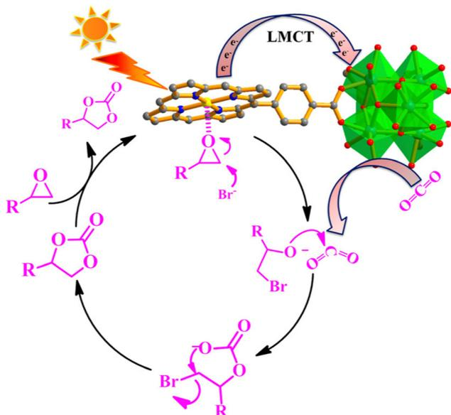
Fig. 22 Mechanism proposed for the PCN-224(Mg)-photocatalysed cycloaddition of epoxide to CO<sub>2</sub>. Reprinted with permission from ref. 239. Copyright 2022 American Chemical Society.
