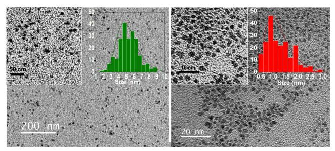
Fig. 1 TEM micrographs of PtFe NPs (left) and PtPt NPs (right) at different magnifications, with their corresponding size distribution charts.
