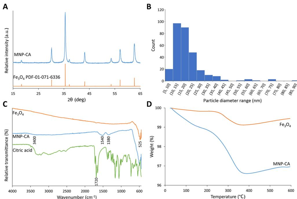
Fig. 2 (A) PXRD patterns of synthesised MNP-CA and pristine Fe<sub>3</sub>O<sub>4</sub> from the powder diffraction file database (PDF-01-071-6336).<sup>50</sup> (B) Histogram showing the size distribution of MNP-CA from TEM image analyses. (C) FTIR spectra for pristine Fe<sub>3</sub>O<sub>4</sub>, synthesised MNP-CA, and citric acid. (D) Graph showing weight loss on heating during TGA for pristine Fe<sub>3</sub>O<sub>4</sub> and synthesised MNP-CA.
