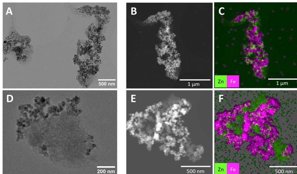
Fig. 6 (A) and (D) TEM images of agglomerate particles of MFC UTSA-16(Zn)@MNP-CA (18.7%), containing both UTSA-16(Zn) and MNP-CA nanoparticles. (B), (C), (E) and (F) TEM EDX images of the MFC showing the distribution of Zn (green) from UTSA-16(Zn) and Fe (pink) from MNP-CA in the agglomerate particles.
