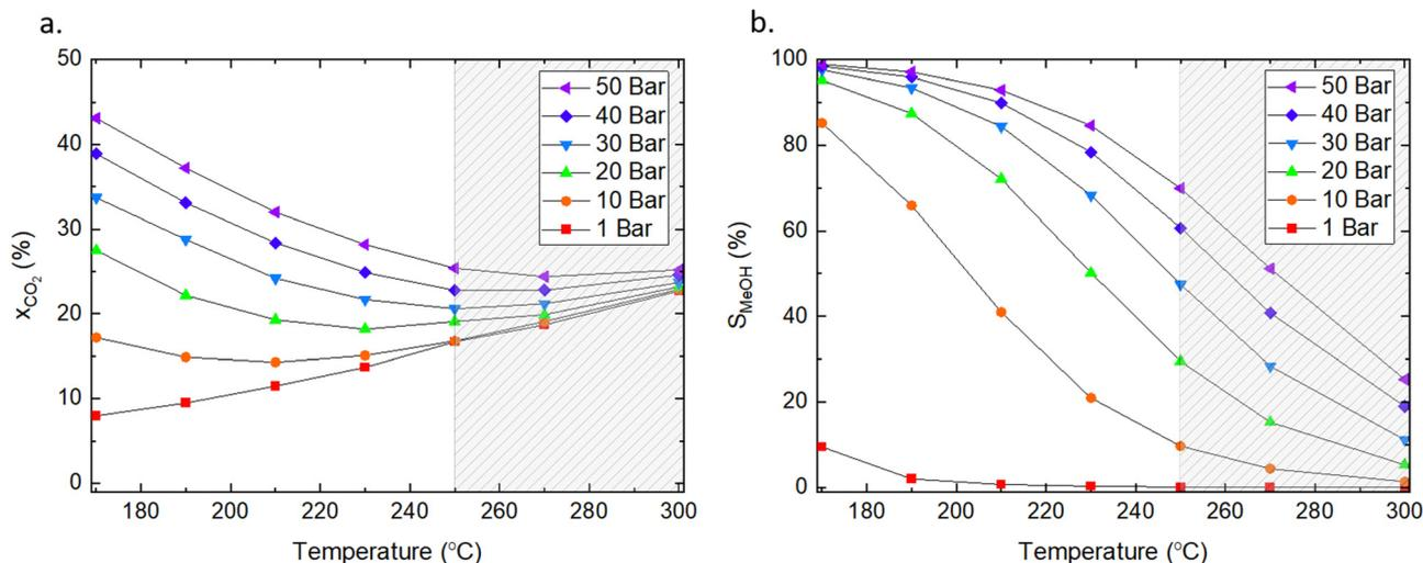
Fig. 2 Influence of pressure and temperature on (a) equilibrium conversion of CO<sub>2</sub> and (b) selectivity toward methanol at equilibrium. The dashed area indicates the temperature range typically applied for CO<sub>2</sub> hydrogenation to methanol in industry. The ratio of H<sub>2</sub>/CO<sub>2</sub> was 3 : 1, and methane was excluded from the calculations. Factsage was used for the analyses.<sup>55</sup>
