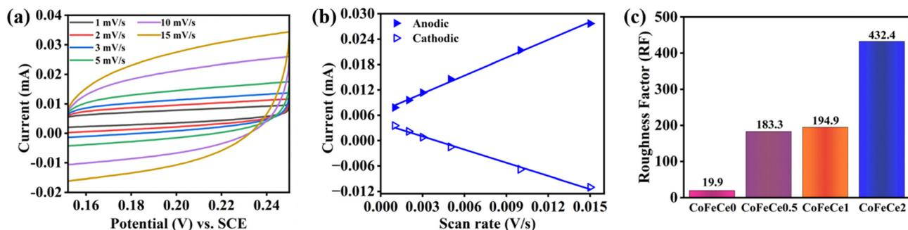
Fig. 7 (a) CVs at different scan rate in a non-faradaic potential region ( $0.15$  to  $0.25 \text{ V vs. SCE}$ ). (b) Plot of anodic and cathodic charging currents at  $0.2 \text{ V vs. SCE}$  vs. scan rate of voltammetry of CoFeCe2 LDH. (c) Roughness factor of Ce-doped CoFe LDHs.
