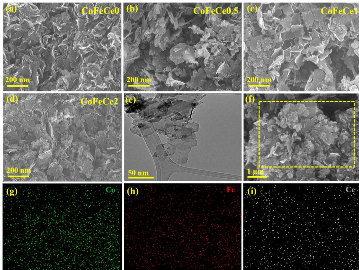
**Fig. 2** Morphological characterization of Ce-doped CoFe-LDHs: (a)–(d) SEM image, (e) a low-resolution TEM micrograph of CoFeCe2 LDH, and (f) SEM image of CoFeCe2 LDH taken for elemental mapping. Elemental mapping for (g) Co, (h) Fe and (i) Ce from the selected area of the SEM image as shown in (f).
