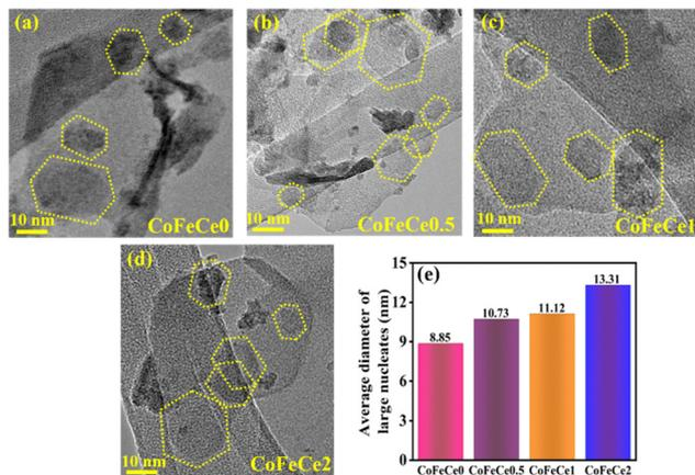
Fig. 5 (a)–(d) HRTEM images of different Ce-doped CoFe LDHs showing large nucleates (dotted yellow line), and (e) bar graph showing the trend in the average diameter of large nucleates in different LDHs.
