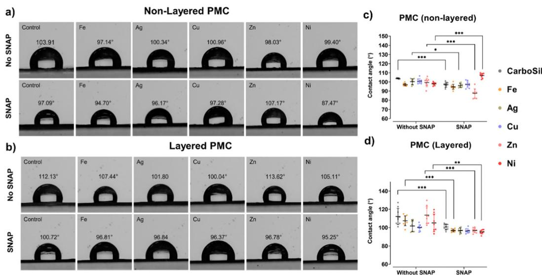
Fig. 4 Contact angle of (a) and (c) non-layered and (b) and (d) layered PMC. Significance is indicated by asterisks where \* is  $p < 0.05$ , \*\* is  $p < 0.01$ , \*\*\* is  $p < 0.001$ . Data is represented as mean  $\pm$  standard deviation.  $N \geq 3$ .
