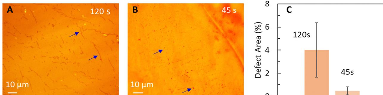
Fig. 2 Optical images of graphene transferred to Nafion (N211) via hot-press ( $\sim 140$  °C,  $\sim 200$  psi) for (A) 120 s, and (B) 45 s. Blue arrows indicate spot like defects that correspond to damages in graphene via oxidation of Cu. Hot-press for longer duration leads to line like larger features (A and Table 1) corresponding to Cu oxidation and damage to graphene. (C) Comparison of % defect area for different hot-press times.
