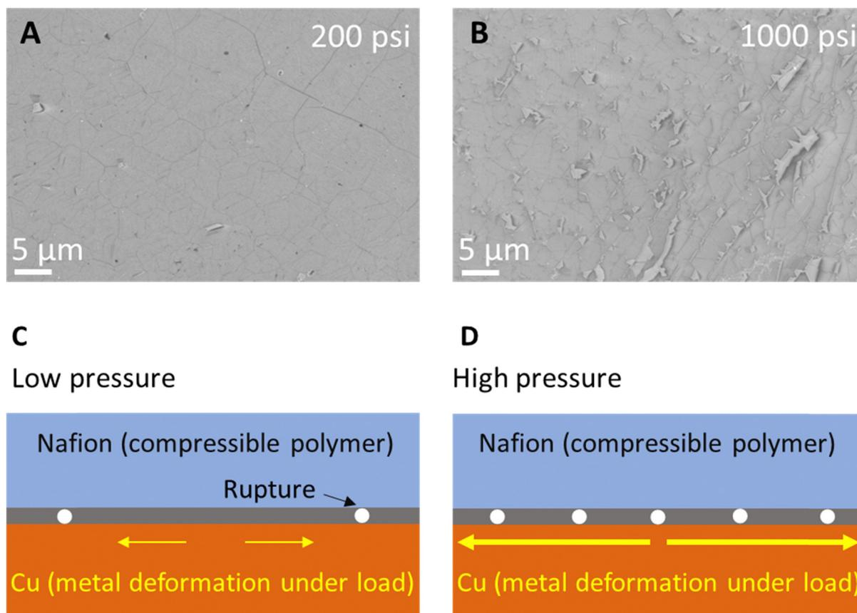
Fig. 4 Graphene transfer on Nafion at  $115\text{ }^{\circ}\text{C}$ , hot-pressed at pressures (A) 200 psi, (B) 1000 psi for 45 s. (C) and (D) At higher pressure the ruptures in the transferred graphene increase due to increase in metal deformation of the Cu foil (note Cu is a soft and malleable metal which is subject to deformation/elongation under pressure). Such metal deformation results in ruptures to the graphene on Cu (see schematics).
