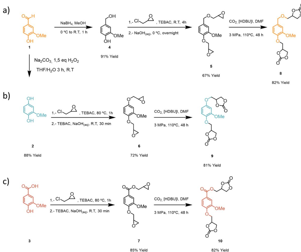
**Scheme 1** Synthetic route for the synthesis of functional bis-carbonates derived from vanillin: (a) vanillin alcohol-based bis-carbonate, (b) hydroquinone-based bis-carbonate, and (c) vanillic acid-based bis-carbonate.
