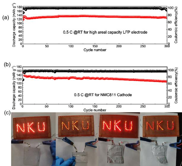
**Fig. 6** (a) Cycling performance and CEs of the Li/rQPE/C-LFP cell at a current density of 0.5C. (b) Cycling performance and CEs of the Li/tQPE/NMC811 cell at a current density of 0.5C. (c) Digital photos of the Li/rQPE/LFP pouch cell under different states: flat, folding, nail penetration and cutting into pieces, respectively.
