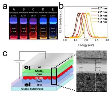
**Fig. 16** (a) Toluene dispersion of decane: SiQDs synthesized from disproportionation reaction of TES under 365 nm UV light irradiation, (b) PL-emission of toluene dispersion of different size SiQDs, and (c) potential arrangements of SiQD-LED and TEM image of sandwich layers. Adapted with permission from ref. 139. Copyright (2020) American Chemical Society.
