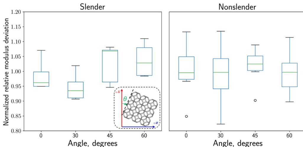
**Fig. 6** Angle-based stiffness trends. The printing angle, measured from the vertical, determines the amount of “stair-stepping” due to the layer-based fusion process. To isolate the effect of printing angle, measured stiffness values are normalized relative to predicted values obtained using the empirical scaling relationships for each specimen. Results are grouped based on slenderness; slender lattices have a relative density less than 10%.
