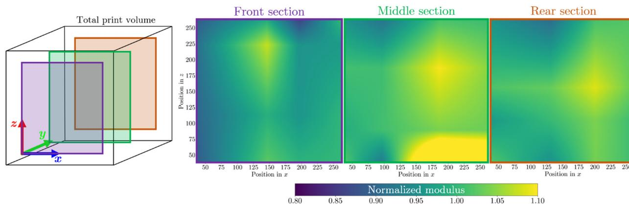
Fig. 5 Location-dependent stiffness for a build volume containing tessellated specimens of the same geometry (Kelvin lattice). Stiffness values are normalized to the cohort average. Panels on the right show linearly interpolated data for various  $y$ -slices (see schematic at left), illustrating the variability of stiffness as a result of location-based differences in part cooling trends.
